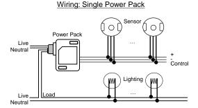
The PS-112 / PS-124 power pack supplies DC power to low voltage occupancy sensors and receives input from the sensor to control a wide range of load types, including lighting or HVAC devices.
